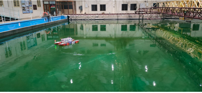
FIGURE 4: Free running test in wave basin
