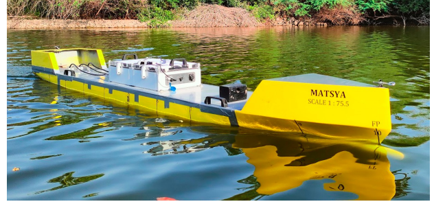
FIGURE 1: Free running model equipped with sensors
