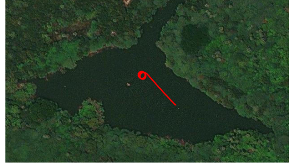
(a) Port side turning circle maneuver GPS plot
