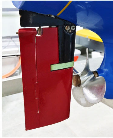
Figure 3: Rudder and propeller outfitted on the vessel
