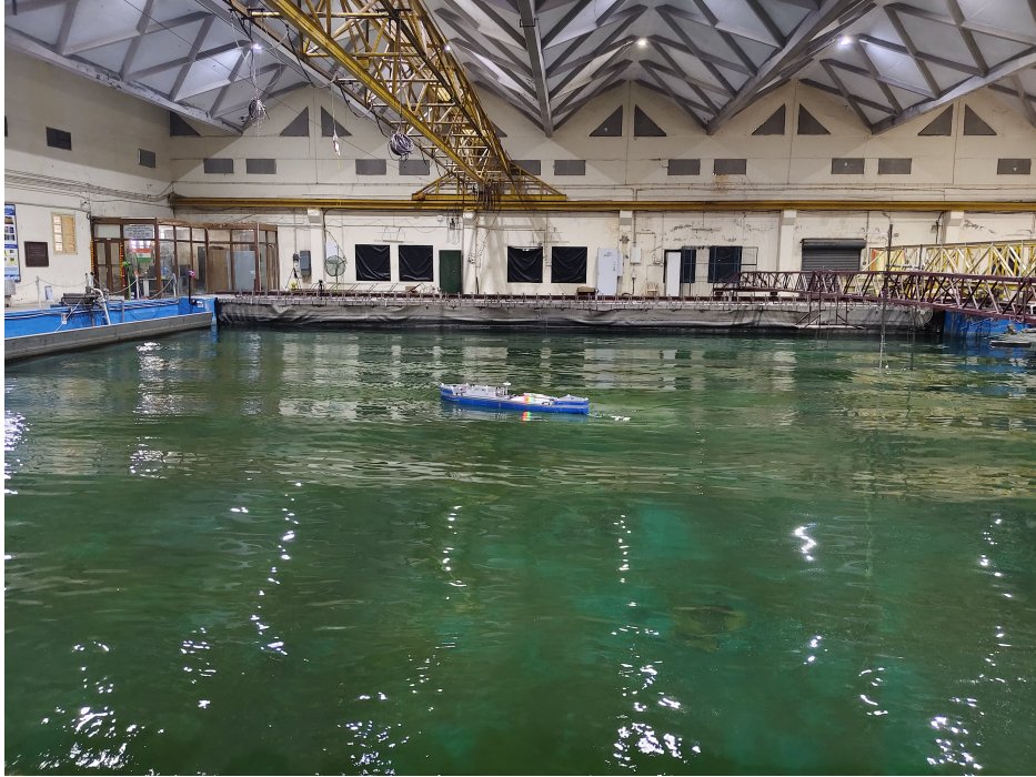
Figure 4: Vessel experiencing waves in the wave basin
